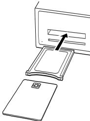
To watch **Conax-scrambled** pay channels, insert a **Conax pay-TV** card into the card slot. To watch non-Conax channels, insert a **pay-TV** card into a CA module, and then insert the **CA** module into the **CAM** slot.
